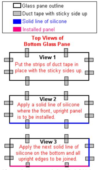
After each glass pane is installed, fold the 2 pieces of bottom duct tape upward, and wrap 2 additional pieces around the corner from one side to the other, as shown below.
